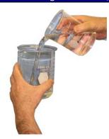
PSF-10cSt Dielectric Silicone Fluid is an excellent choice for systems that require a low viscosity fluid and high dielectric strenath.
